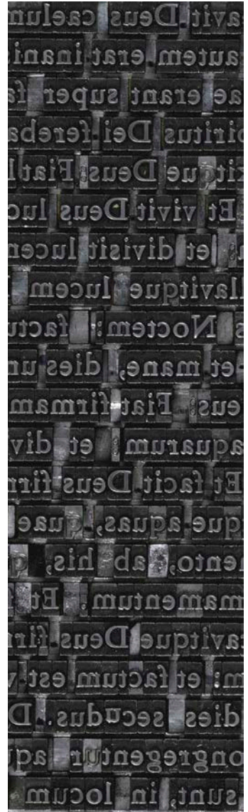
Above: Detail of metal type locked in a printing form. The text is from Genesis 1 in the Latin Bible.
